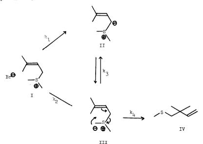
When **8**, **8**-dimethylallyldimethylsulfonium bromide(I) was treated with n-butyllithium in hexane-tetrahydrofuran at -78° and the reaction mixture warmed to 0° for workup, the homoallyl sulfide IV, isomeric with the desired ylide II, was isolated in 84% yield. The struc-
